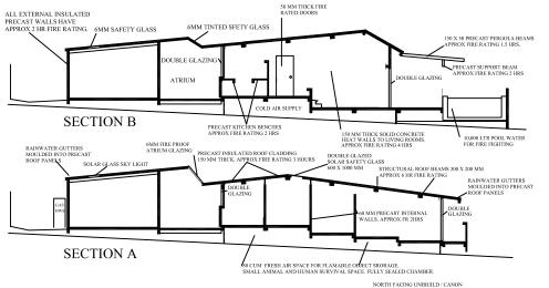
A FIRE RATING IS A FIRE TEST TO DESTRUCTION. THIS MAY TAKE 2 OR MORE HOURS OF CONSTANT FLAME. A TYPICAL BUSHFIRE PASSES THROUGH IN ONLY MINUTES. THIS NON FLAMABLE STRUCTURE WILL NOT BURN DURING THE PASSAGE OF THE FIRE STORM.
